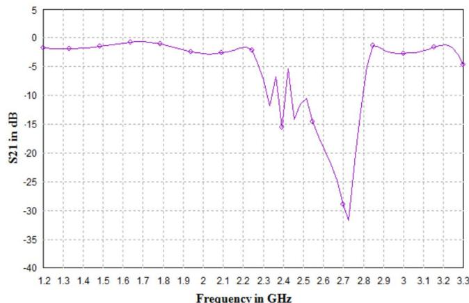
Figure 3. Band gap analysis of EBG
