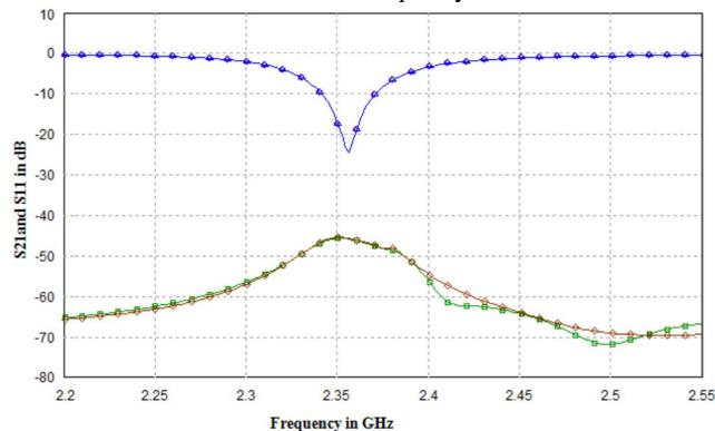
Figure7. H-plane coupled microstrip antennas separated by EBG structure with patch size  $25\text{mm}$
