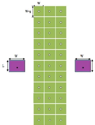
Figure 1. EBG structure integrated with microstrip patch antenna array to reduce mutual coupling
