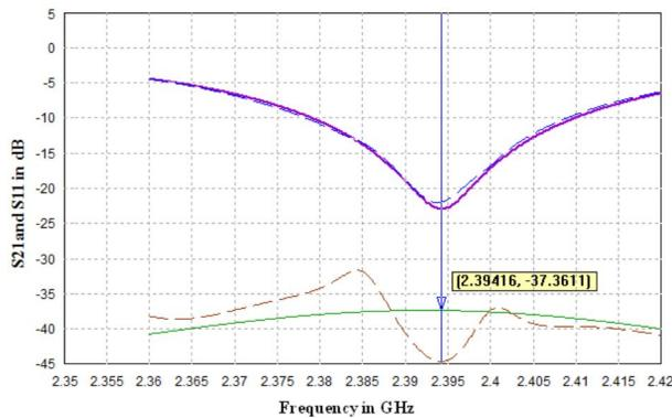
Figure 6. Measured results of microstrip antennas with and without the EBG structure. An  $8\text{dB}$  mutual coupling reduction is observed at resonant frequency
