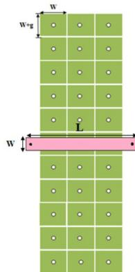
Figure 2. EBG simulation model
